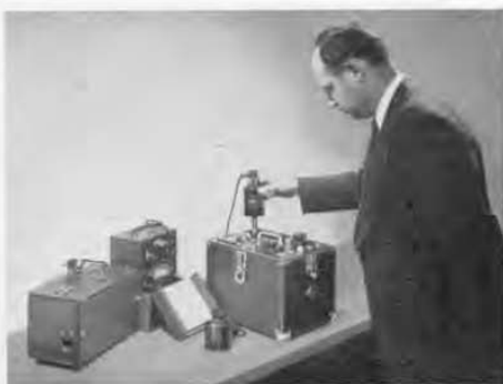
Figure 5. Calibrating a sound-level meter with the sound-level calibrator. A Type 723-B Oscillator and Type 727-A Vacuum-Tube Voltmeter provide the standard 400-cycle voltage.
